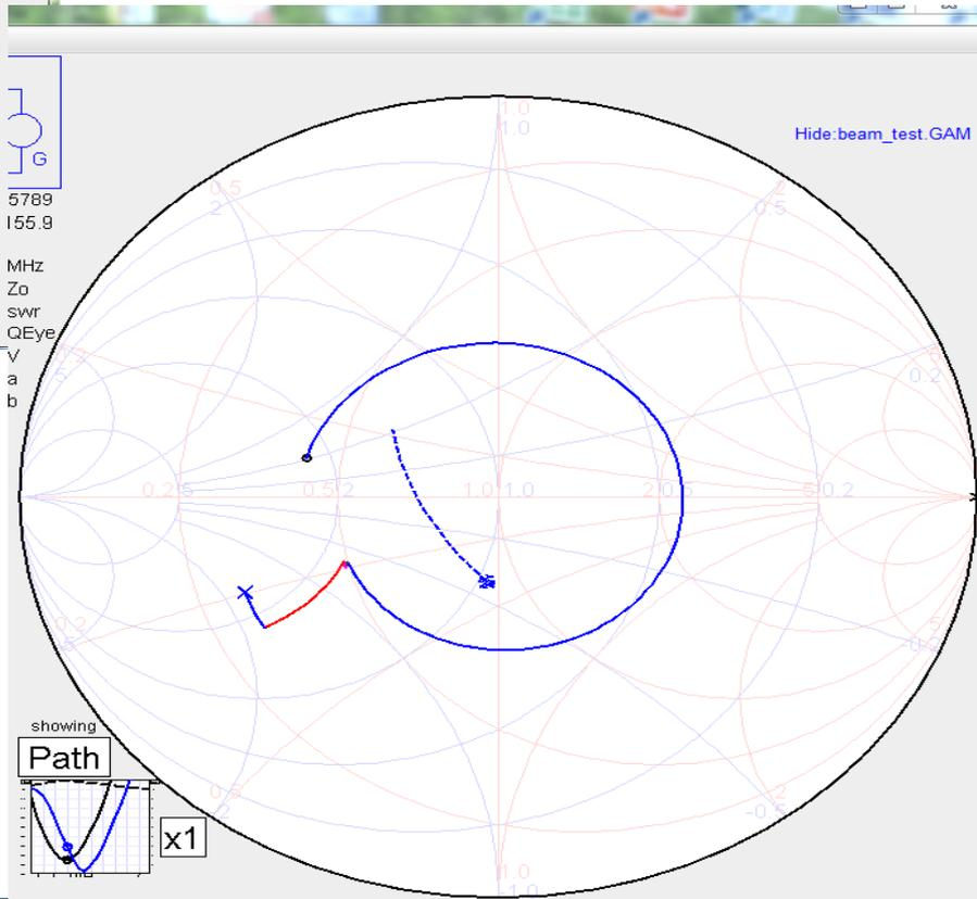
Above is plot of VSWR at transmitter end and load end with antenna tuner in line.
