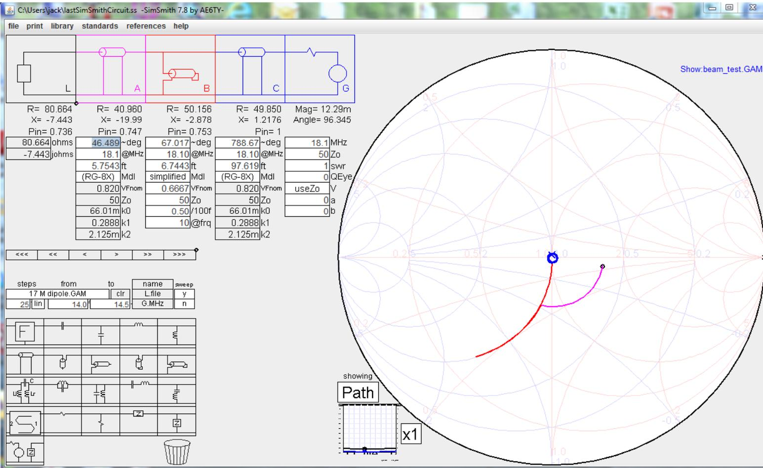
SimSmith Transmission line modeling with input from antenna modeling can model entire systems
